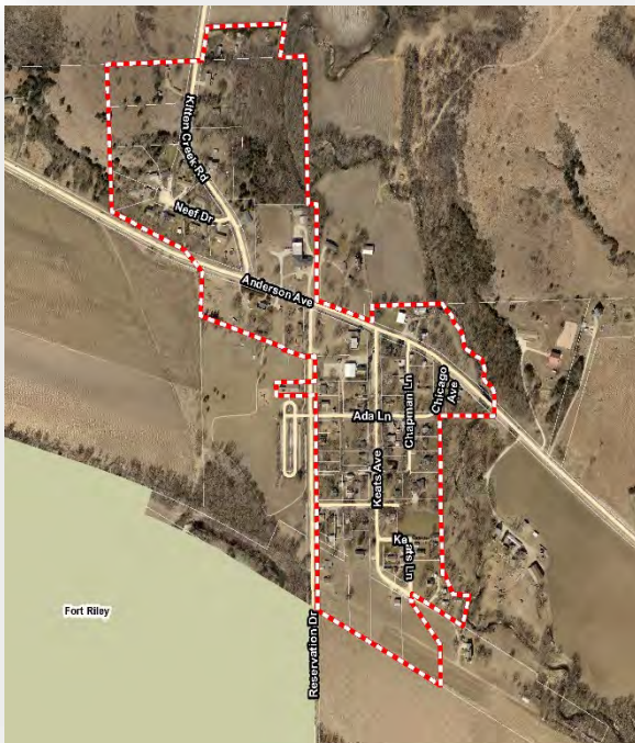
Figure 19 The Potential Keats Sewer District, outlined in red, will help alleviate environmental concerns caused by septic tanks in the area.
